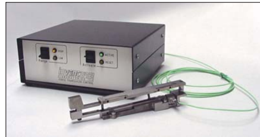
Inventure Laboratories Force Transducer (above) provides a cleaner, more accurate signal than the original T.M. Long force transducer, compared below.
