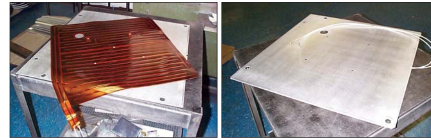
Inventure Laboratories replacement plate heaters are more efficient and heat more uniformly than the original T.M. Long heaters. The heating element (left) is encased in the plate housing (right).
